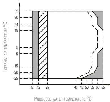
■ Operating range with heat pump with possible limitation and protection
