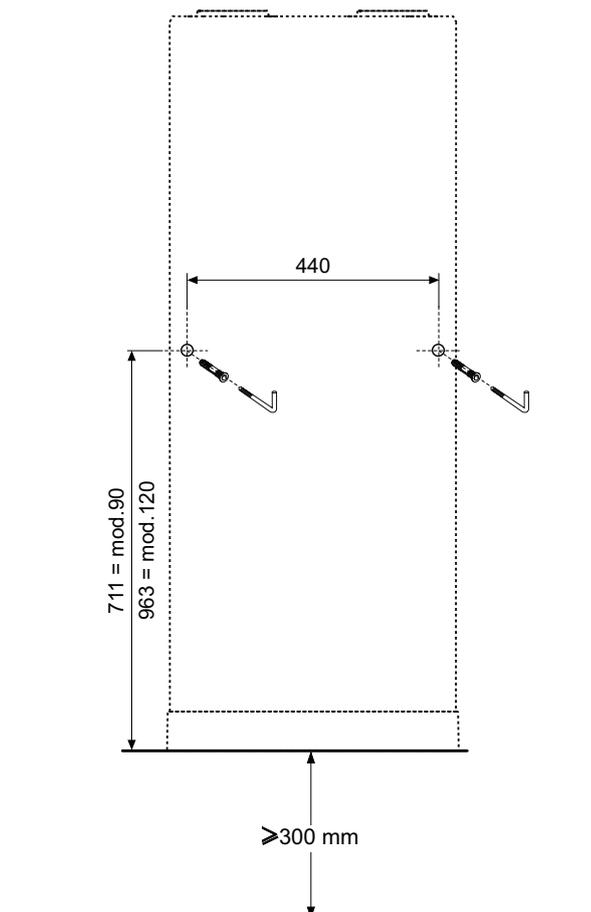
fig. 50 - Drilling indication
