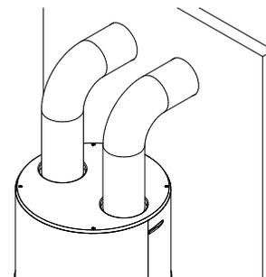
fig. 52- Arrangement of air channels
