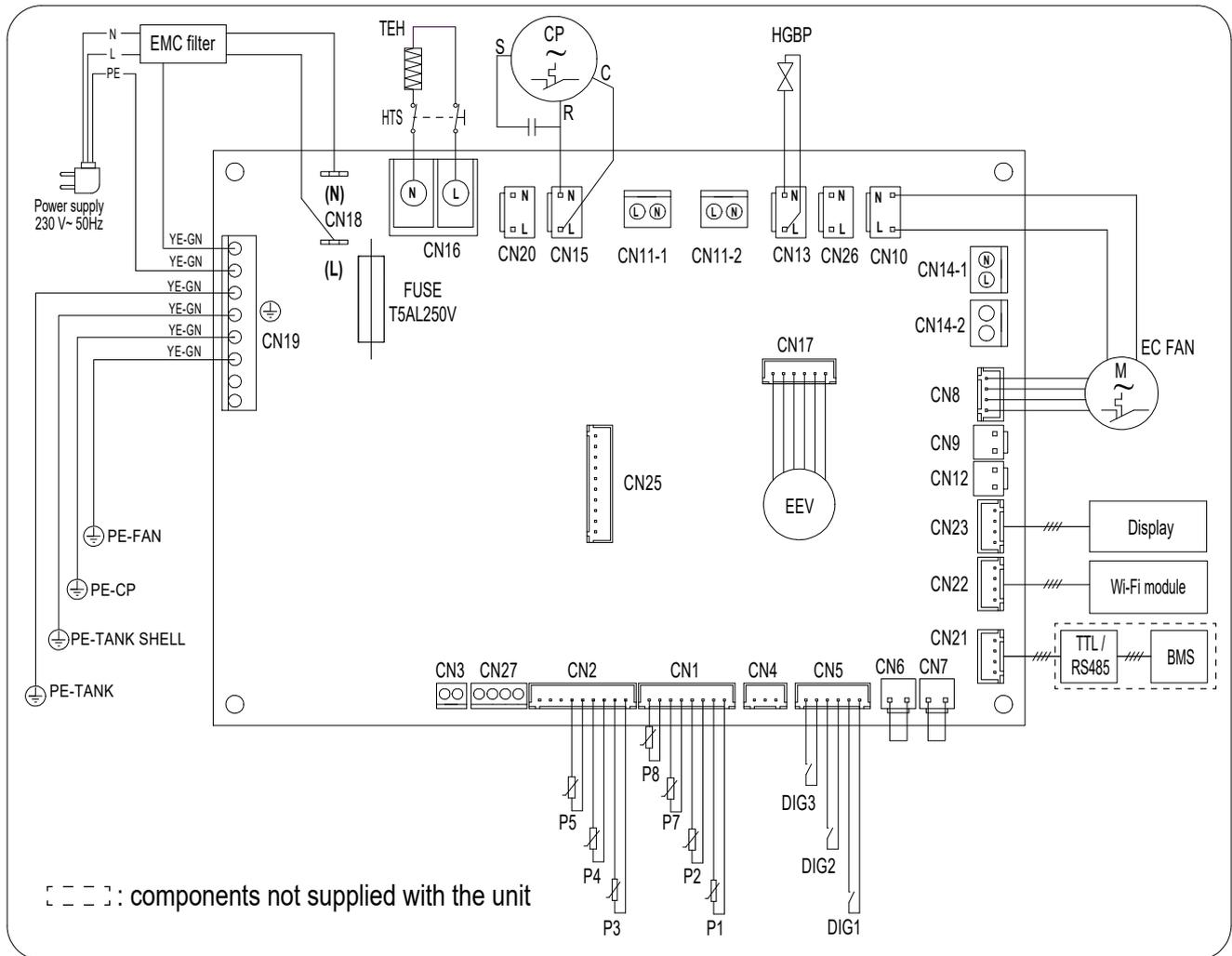
fig. 63 - Wiring diagram of the equipment
