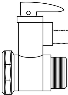
fig. 55 - Safety valve 0.7 MPa (7 bar)
