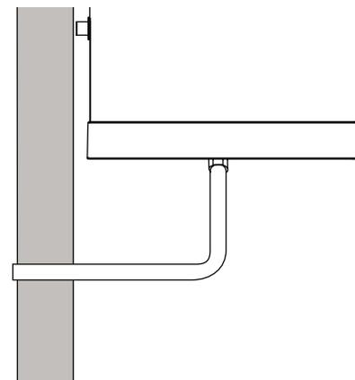
fig. 57- Example of condensate drain connection without a trap
