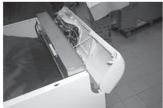
Fig. 6 - Turn the control panel forwards.
